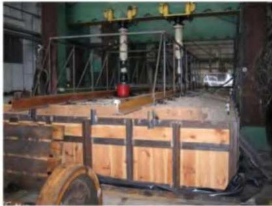
Figure 3.14. View of the testing stand for a new type of railway track [129].
